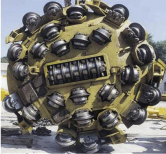
Fig. 9. Cutters position on cutter head of 3.6 m diameter.
