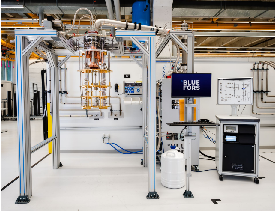
Figure 1.2: The image shows a dilution refrigerator produced by Bluefors. The depicted refrigerator is unshielded, revealing its internal structure. Source: Bluefors.
