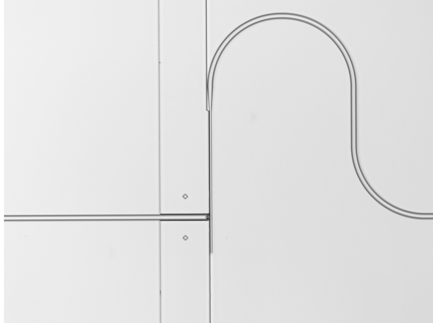
Figure 6.6: The image presents a microscopic view of the flux bias line and the resonator end grounded through the DC-SQUID.
