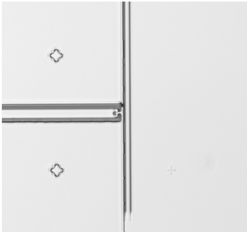
Figure 6.7: The image presents a detailed microscopic view of the flux bias line and the DC-SQUID.
