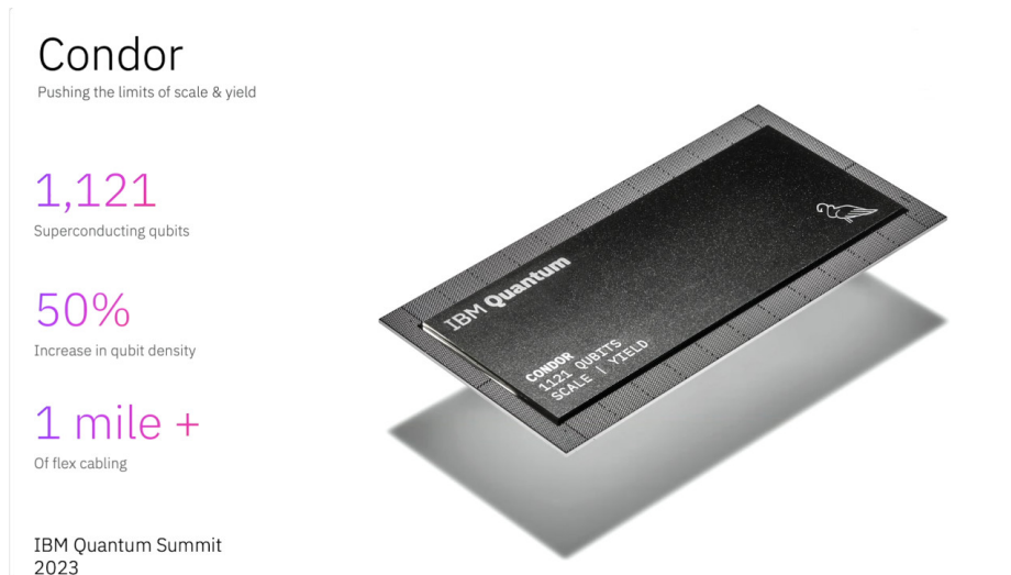
Figure 4.1: 1121-Qubit chip produced by IBM: This chip not only contains an array of qubits but also includes resonators and control lines essential for qubit operation. Source: IBM.
