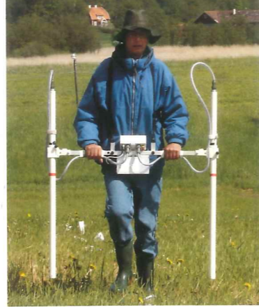
The Bartington Grad601-2 single-axis, vertical-component, high-stability fluxgate gradiometer system.
