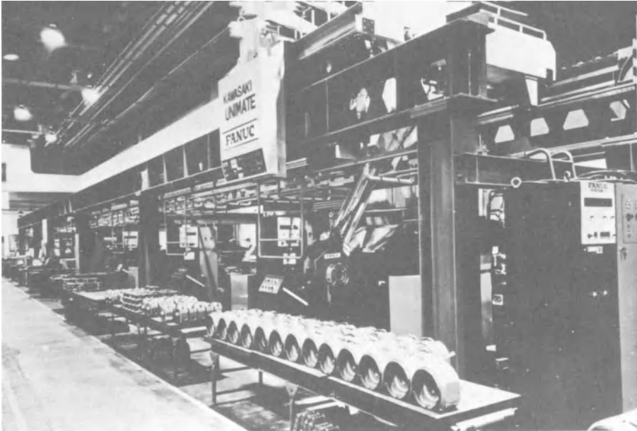
Figure 4.8 Robot travels to work – overhead robot serving eight NC lathes
