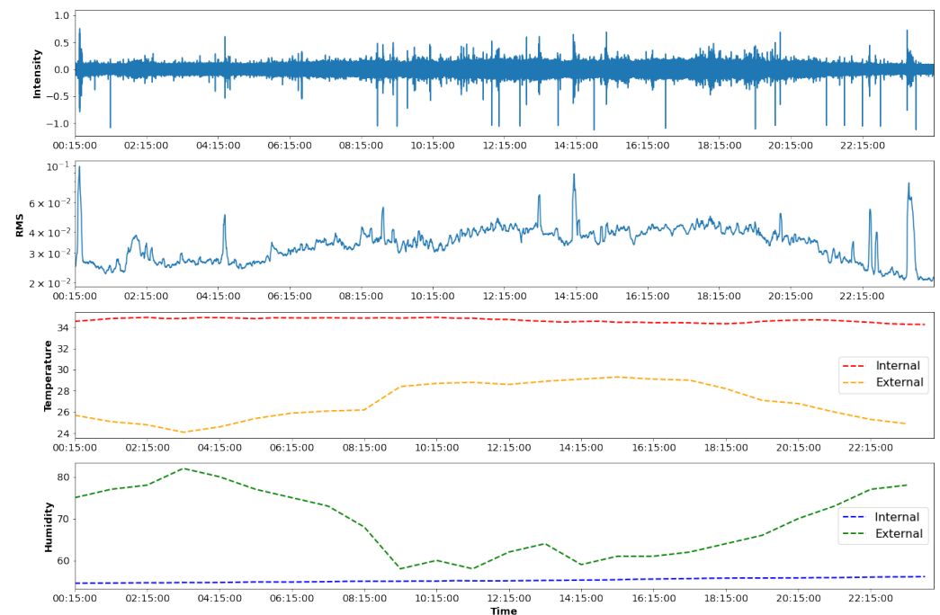
Figure 2. Time series, from top to bottom, of audio intensity, audio RMS, internal/external temperature, and internal/external humidity readings in a hive with 3 boxes and 30 full frames of bees (date: 12 August 2021).
